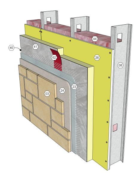
Adhered stone veneer over steel studs backup, rigid insulation w/ taped joints Wall 03.080.0203 Rev. 11/23/15
