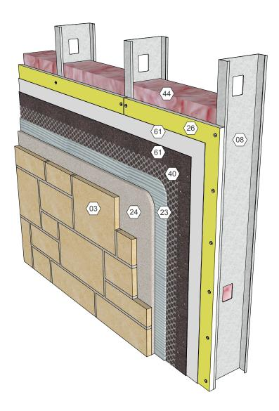
Adhered stone veneer over steel studs backup, fiberglass insulation
