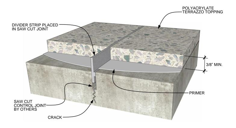
POLYACRYLATE TERRAZZO DIVIDER STRIP PLACED IN SAW CUT CJ
