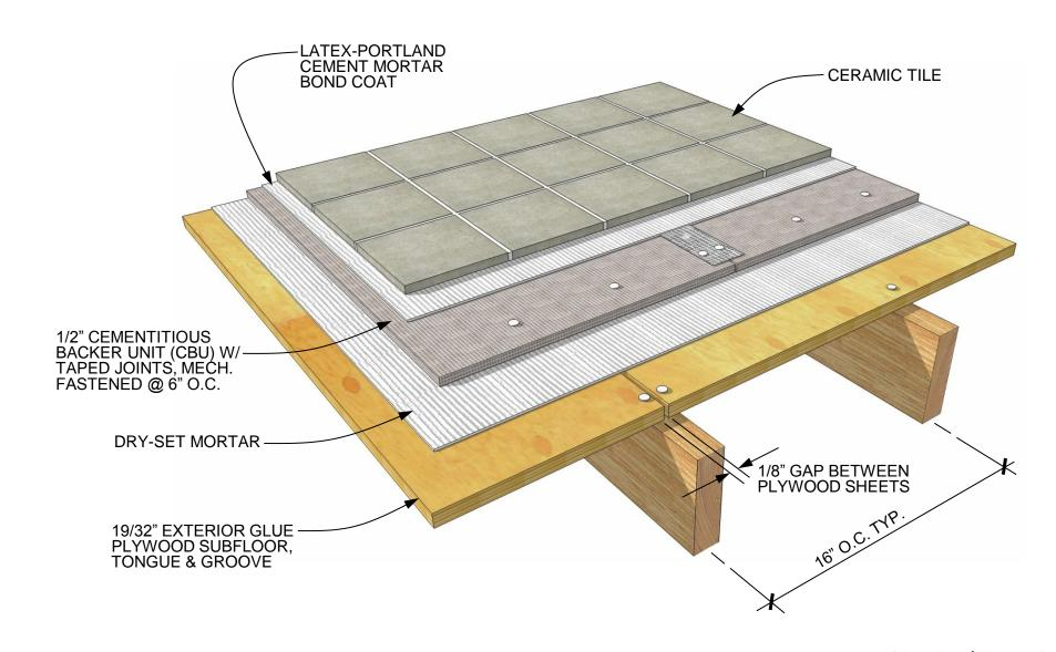
FLOOR TILE OVER CBU ON WOOD SUBFLOOR DETAIL 06.130.0101 REV. 08/31/09
