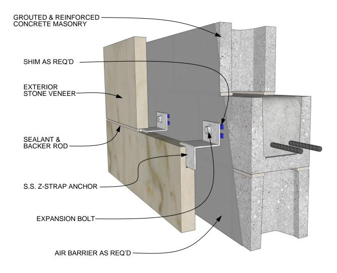
EXTERIOR STONE RESTRAINT ANCHORAGE Z-STRAP ANCHOR
