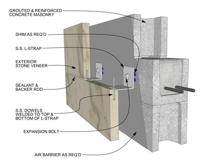
EXTERIOR STONE RESTRAINT ANCHORAGE
