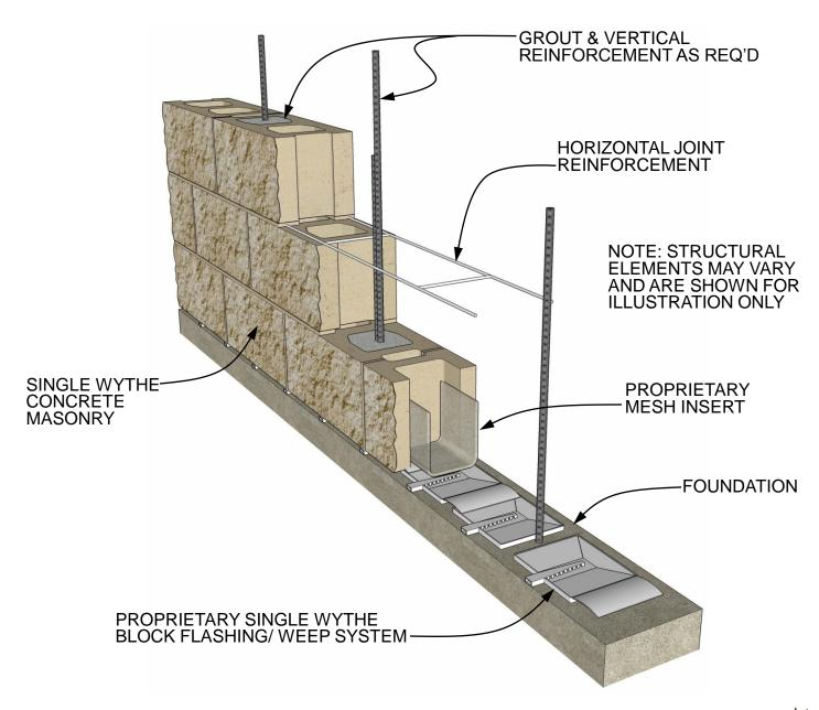
BASE OF WALL SINGLE WYTHE BLOCK, PROPRIETARY FLASHING/WEEPS
