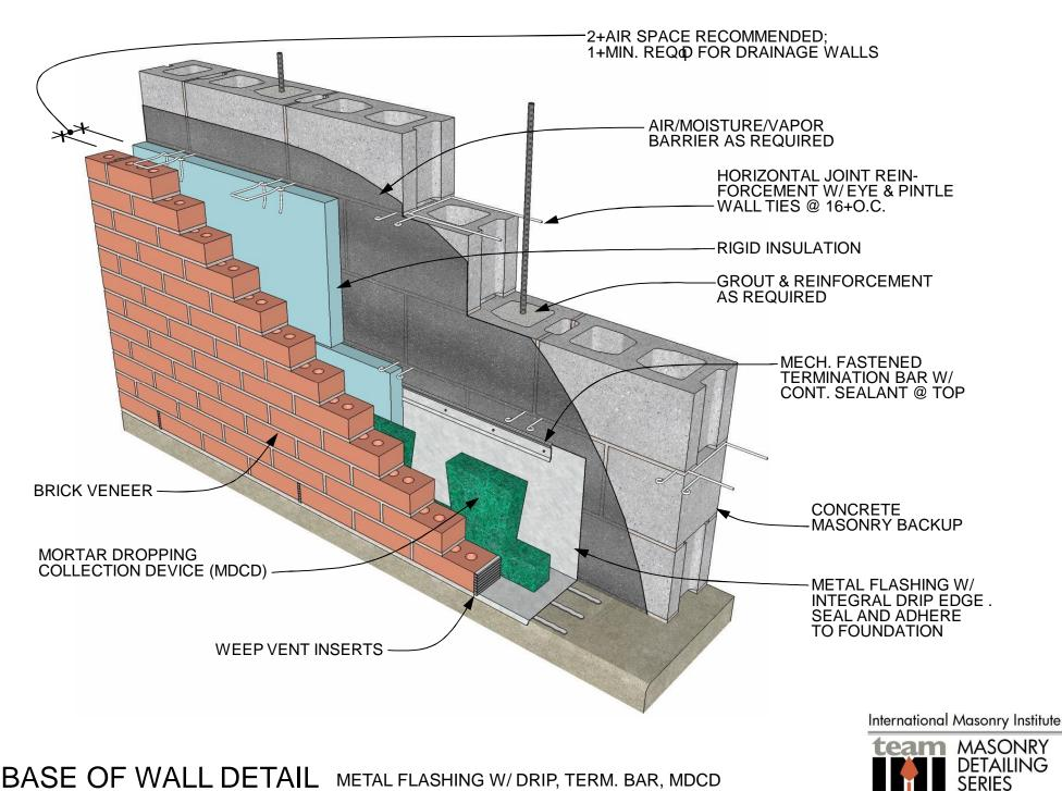
BASE OF WALL DETAIL METAL FLASHING W/DRIP, TERM. BAR, MDCD
