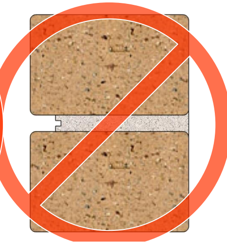
3. JOINT GROUND TO INCORRECT PROFILE
