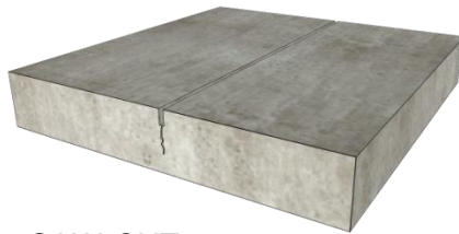
SAW-CUT CONCRETE AT CRACK
