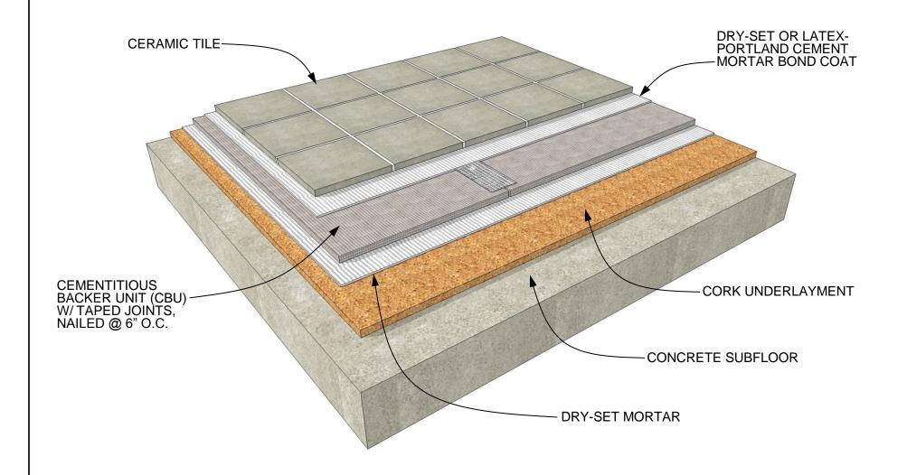
FLOOR TILE OVER CBU & CORK ON CONCRETE DETAIL 06.130.0204 REV. 08/25/09
