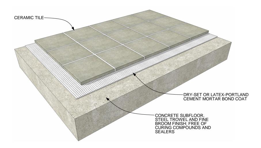
FLOOR TILE THINSET ON CONCRETE DETAIL 06.130.0203 REV. 08/25/09
