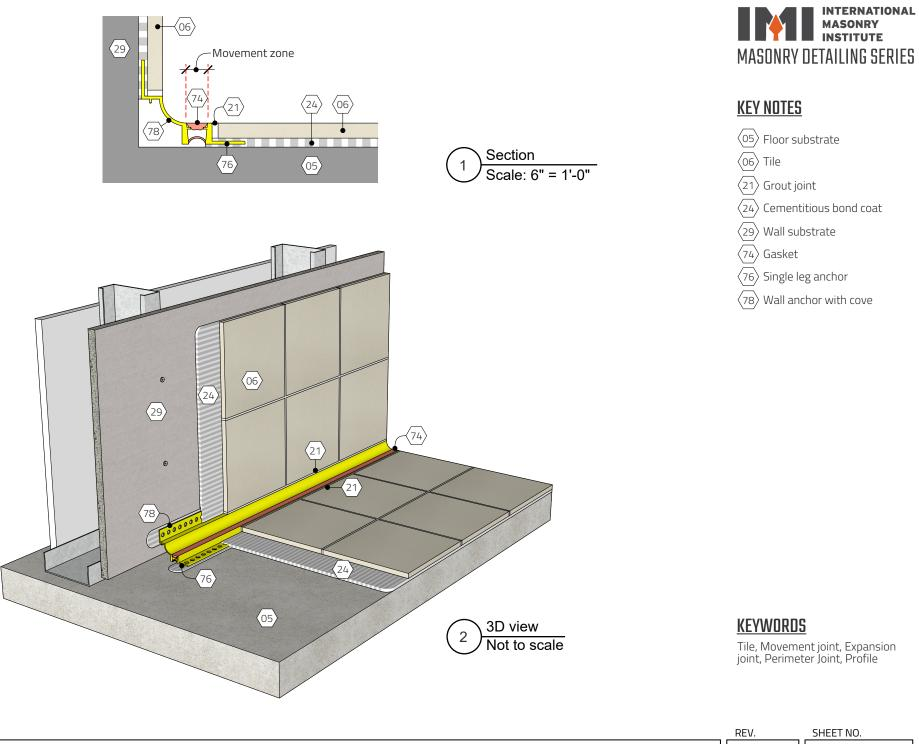
Perimeter Movement Joint Detail - Tile | Prefabricated Joint Profile at Floor-Wall Interface
