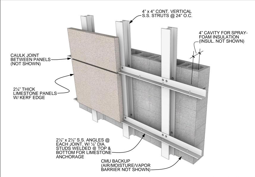
Stone Anchorage Detail – CMU Backing | Steel Struts & Angles
