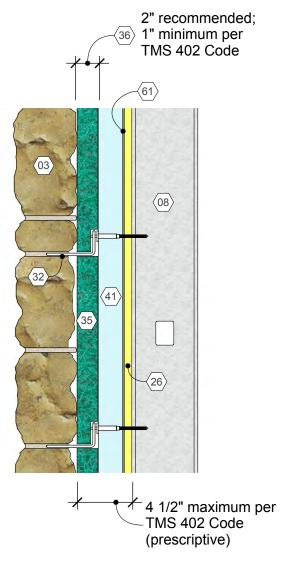
Stone Veneer, Steel Stud Backup Detail 03.040.0201 Rev. 7/28/16
