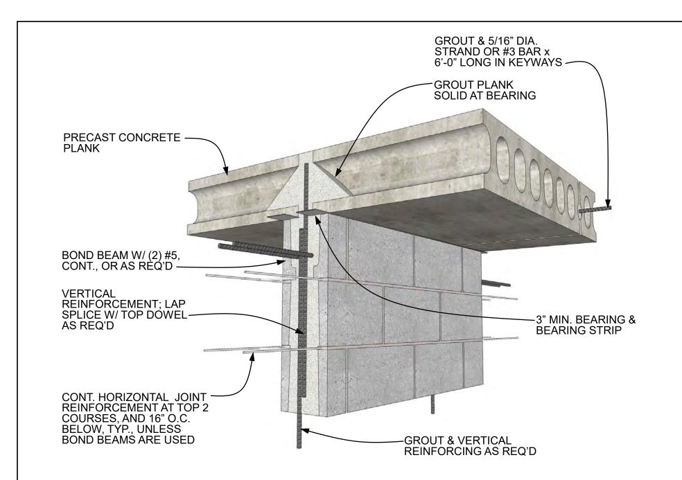
Top of Wall Detail – Single Wythe CMU | Precast Concrete Plank at Bearing Wall DETAIL 02.120.0952 REV. 8/12/24
