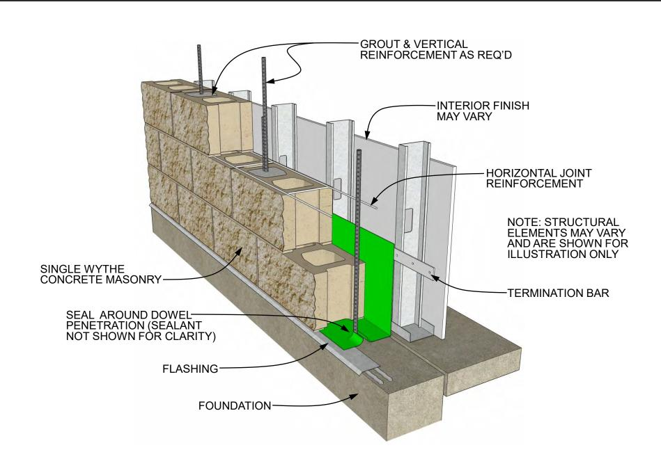
BASE OF WALL SINGLE WYTHE BLOCK, FLASHING @ INSIDE FACE DETAIL 02.010.0312 REV. 06/30/11
