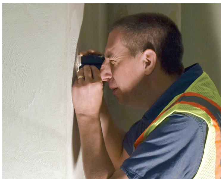
BOB SCORE, RESTORATION ARCHITECT WITH HARBOE ARCHITECTS, PC, EXAMINES THE TEXTURE OF A NEWLY-APPLIED PLASTER FINISH THROUGH A MAGNIFIER.
