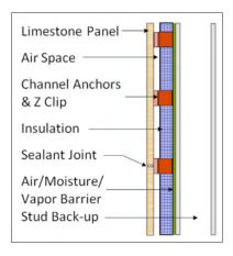
The new applications turned Grande Masonry into an exterior wall specialist, with responsibility for installing the air barrier, Z clips, exterior wall insulation, support channels, stone panels and brick veneer. BAC craftworkers installed the entire exterior wall system. IMI technical support on the details helped ensure
