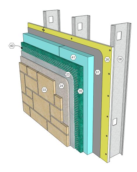
WALL SYSTEM Adhered stone veneer over steel studs backup, rigid insulation, drainage material Wall 03.080.0211 Rev. 11/23/15
