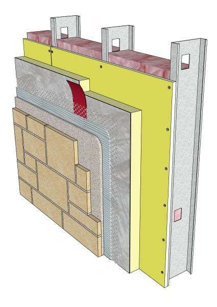
WALL SYSTEM Adhered stone veneer over steel studs backup, rigid insulation w/ taped joints
