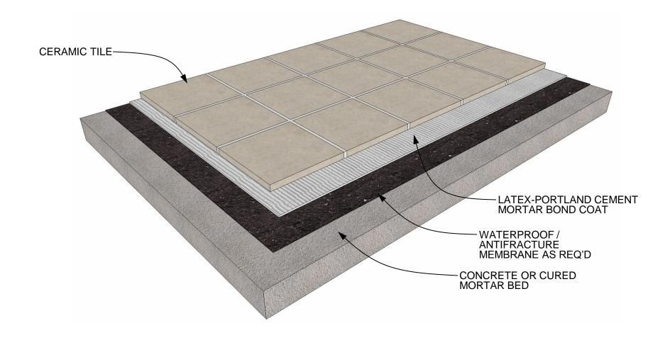
FLOOR TILE THINSET ON CONCRETE OR CURED MORTAR BED DETAIL 06.130.0202 REV. 08/25/09
