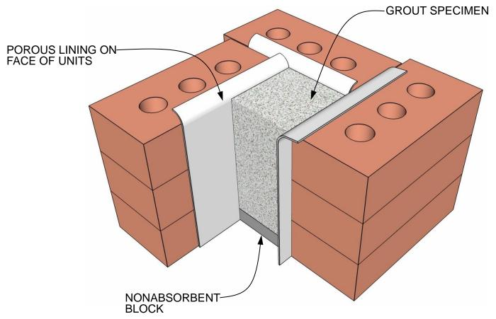
NOTE: FRONT MASONRY UNIT STACK NOT SHOWN TO ALLOW VIEW OF SPECIMEN
