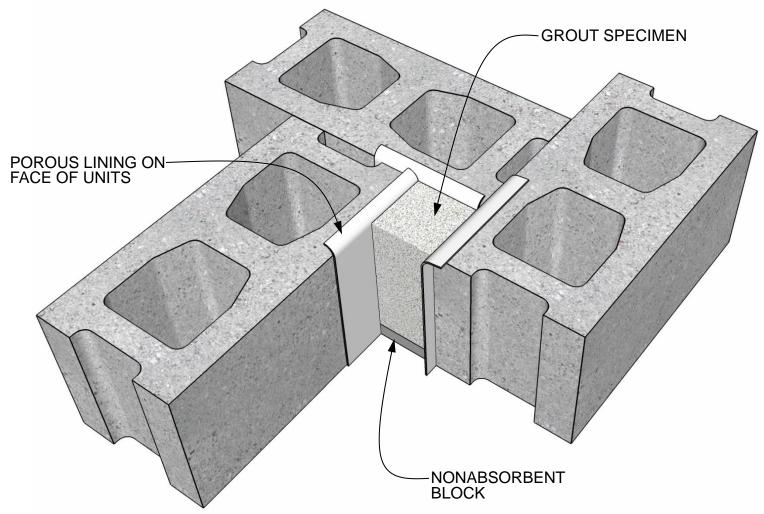
NOTE: FRONT MASONRY UNIT NOT SHOWN TO ALLOW VIEW OF SPECIMEN
