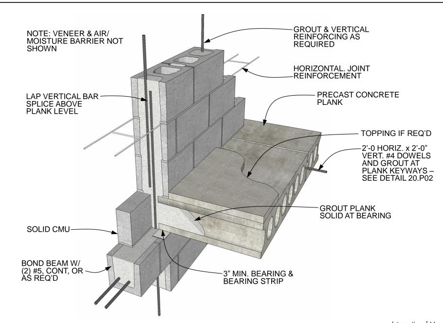
PLANK AT BEARING WALL
