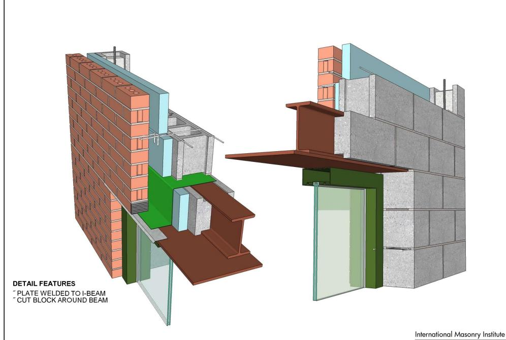
HEAD DETAIL PLATE WELDED TO STEEL BEAM
