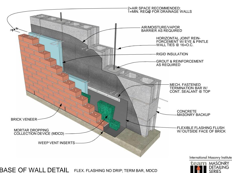
BASE OF WALL DETAIL FLEX. FLASHING NO DRIP; TERM BAR, MDCD
